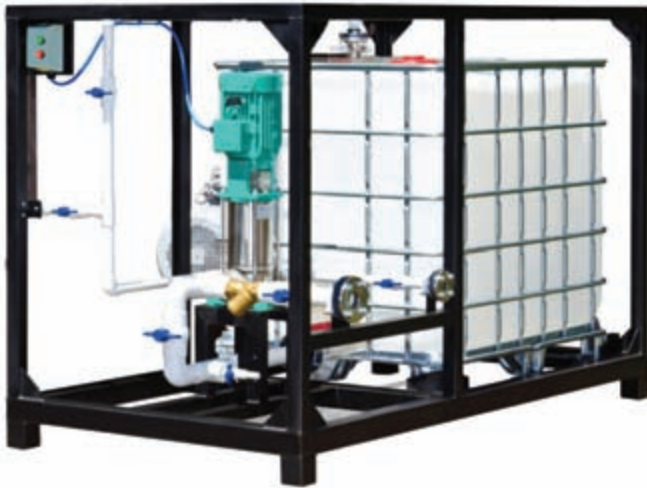
Water phase extension section For UVB-1 1m 3 /hour production capacity
